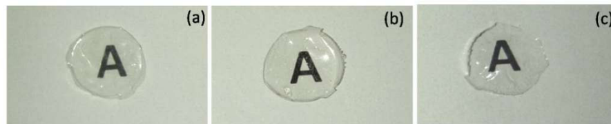
Figure 28. Transparency of RSF films after cell adhesion studies: All the test materials were found to retain its original transparency even after cell culture (a - AQ, b – FA, c – HF).
