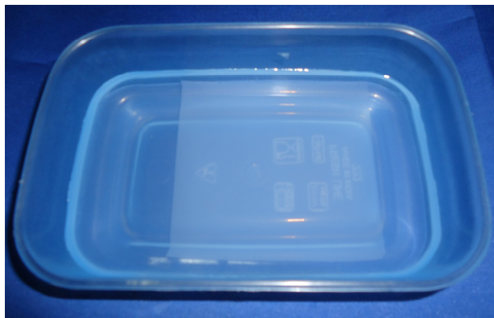
Fig.22: G 200 H 80 Ag sheet with 1mm thickness in PBS.
