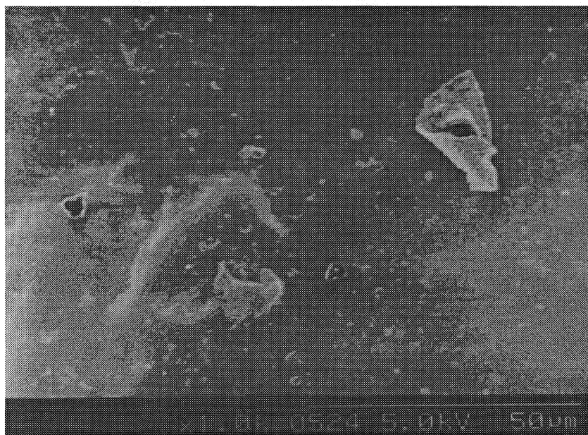
Fig. 3.1.8a SEM of unmodified plasticized PVC sheet
