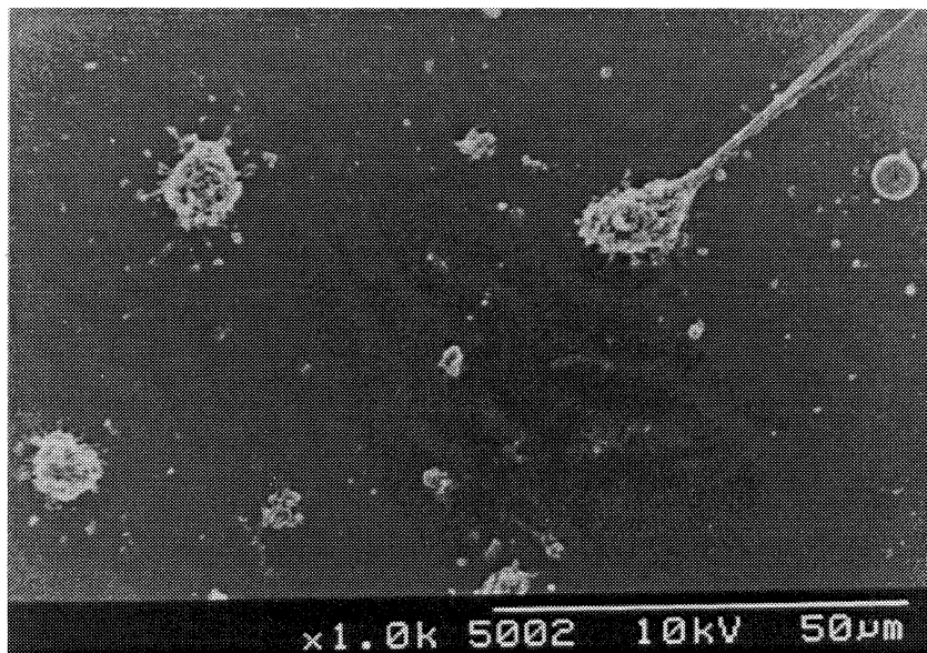
Fig. 3.5.15a SEM of unmodified plasticized PVC tube exposed to human blood for 48 h at 4°C.
