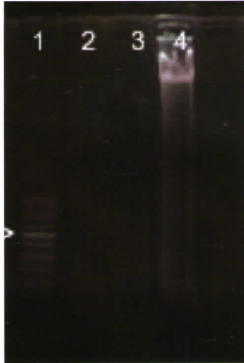
Figure 3-3: 1% Agarose gel showing extractable DNA from decellularised bovine pericardium; 1 st lane: molecular weight marker, 2 nd and 3 rd lane: DNA from decellularised bovine pericardium, 4 th lane: DNA from fresh bovine pericardium (arrow head- 500bp).
