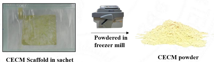
Figure 2. Preparation of CECM powder using a freezer mill
