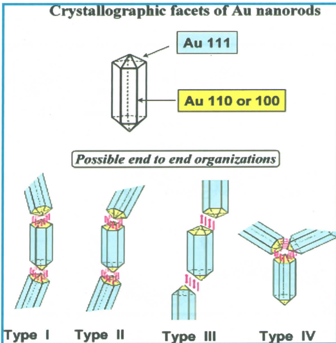
Scheme 2 Crystallographic facets of gold nanorods participating in the gold chain formation (Joseph STS et al.; 2006).
