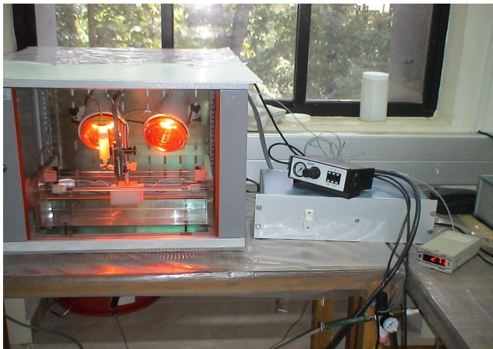
Fig no 3 - Hydrogel Spray coating unit
