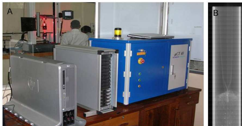
Figure 12: Micro-CT analysis of scaffold: A , micro-CT equipment and B , scout view of sample with container
