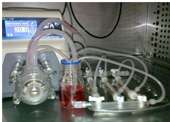
Figure 15: Two channel bioreactor set up for culture of EC and SMC on scaffold
