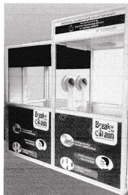
Fig.3. Dual-chamber swab collection booth
