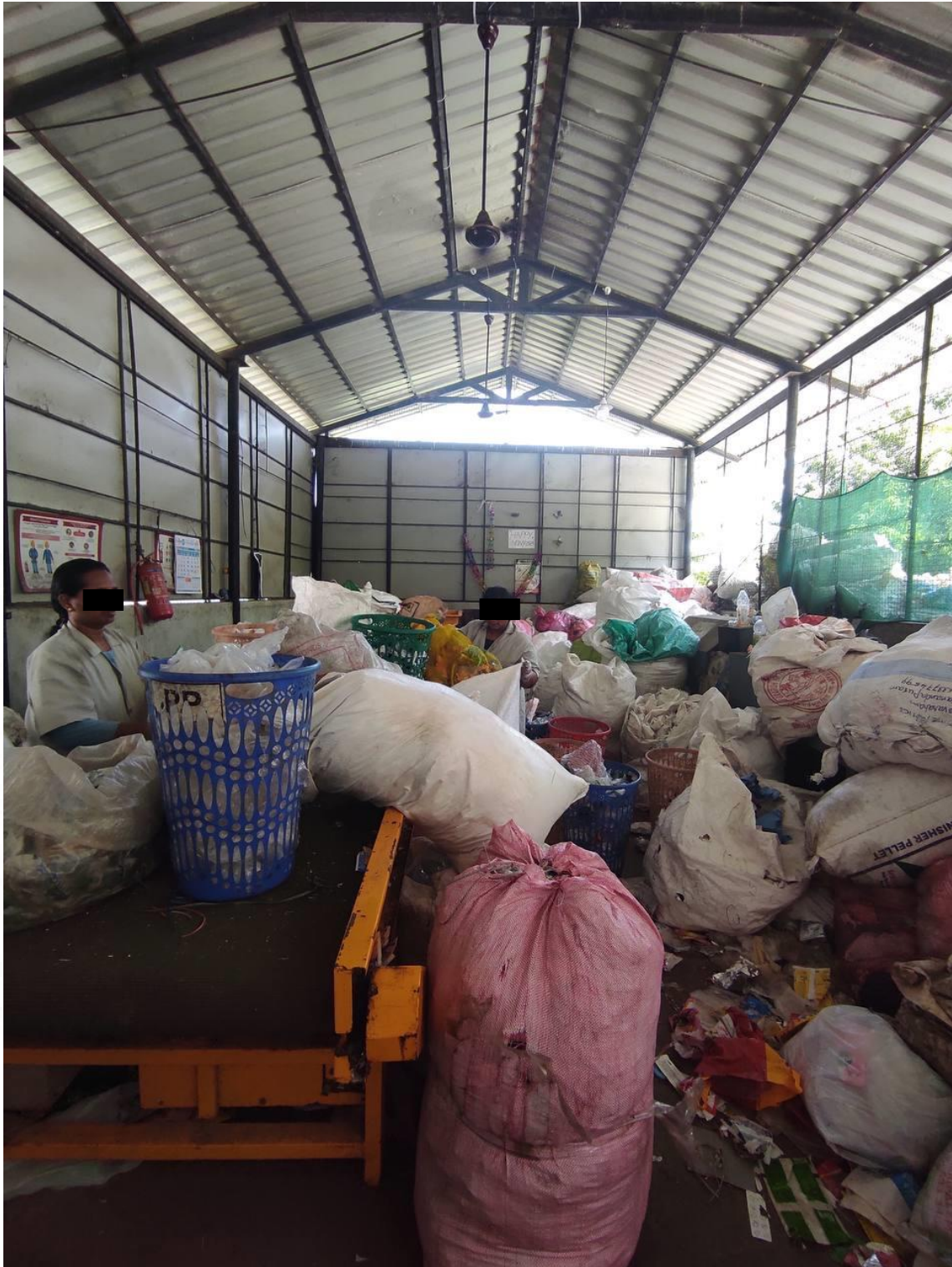
Figure 12: Manual segregation by workers on a non- functional conveyer belt
