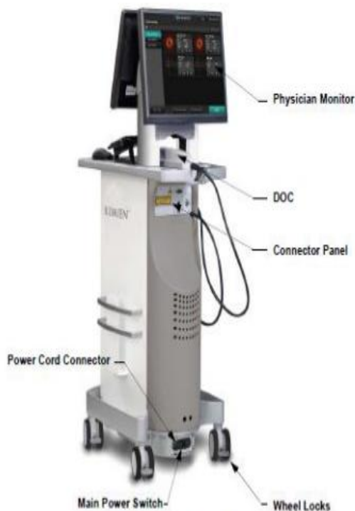
Figure 1-1: ILUMIEN System - Physician Side
