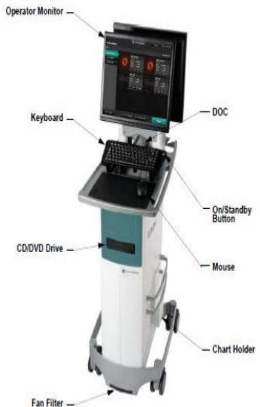
ILUMIEN System - Operator Side
