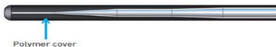
C - Guidewire with polymer cover
