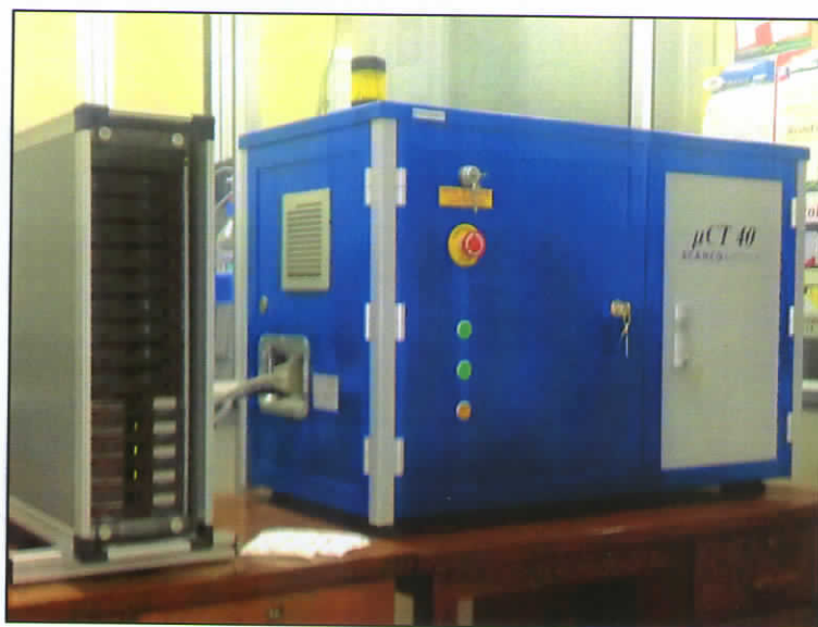
Fig 3: X-ray microcomputed tomography instrument (Scanco \mu CT 40)
