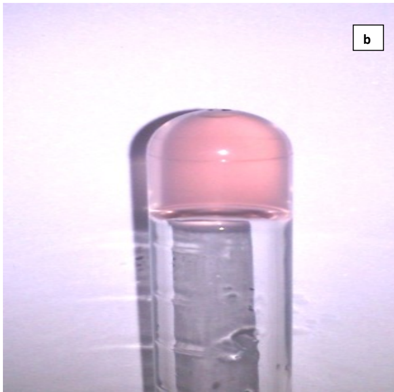
Fig 6. Free flowing pregel formulation (a), gel formed after crosslinking (shown in the inverted tissue culture tube) (b).
