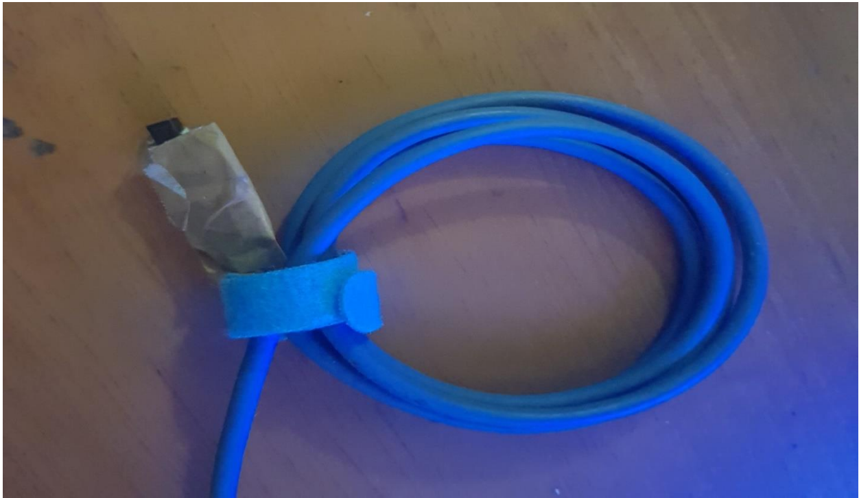
Figure17: This is the temperature sensor for measuring real time data
