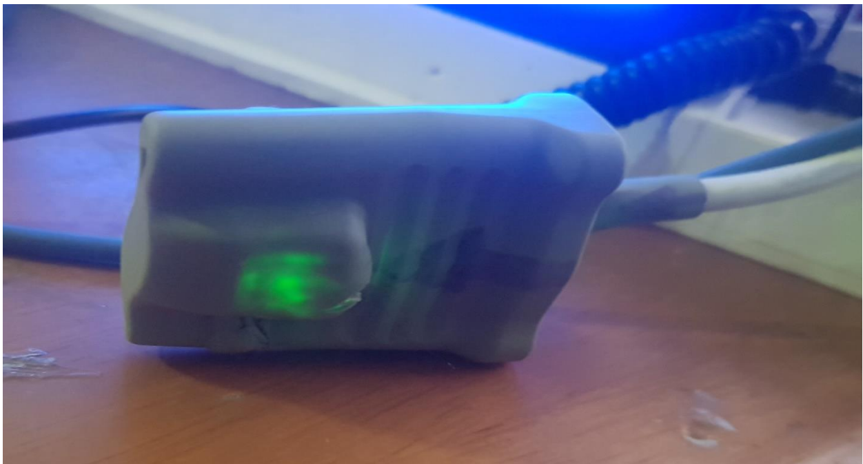
Figure18: Pulse Oximeter sensor with LED lights. The black arrow on the right side is where the finger tip is inserted for measurement.
