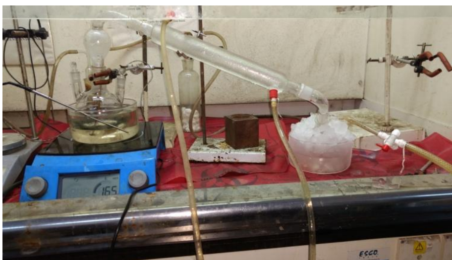
Figure 3.1. Vacuum distillation of 2-hydroxyethylmethacrylate
