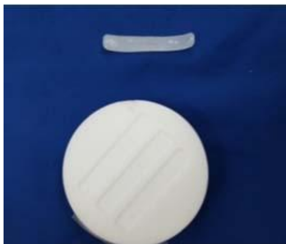
Figure 3.5. Teflon mould for casting polymers and the cast polymer strip
