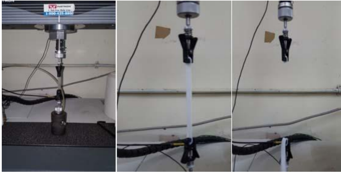
Figure 3.6 Tensile property evaluation using UTM
