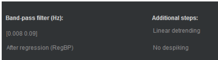
Figure 17: Default settings of Band-pass filter( the value at which effect of confounds can be further reduced and to limit the subsequent connectivity), RegBP(assuming that the effects of regressors are independent of frequency), with linear detrending and no despiking.
