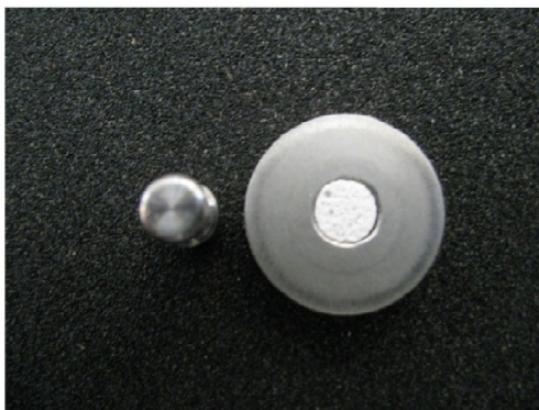
(B) Top Down view Scaffolds in Stainless Steel Mold
