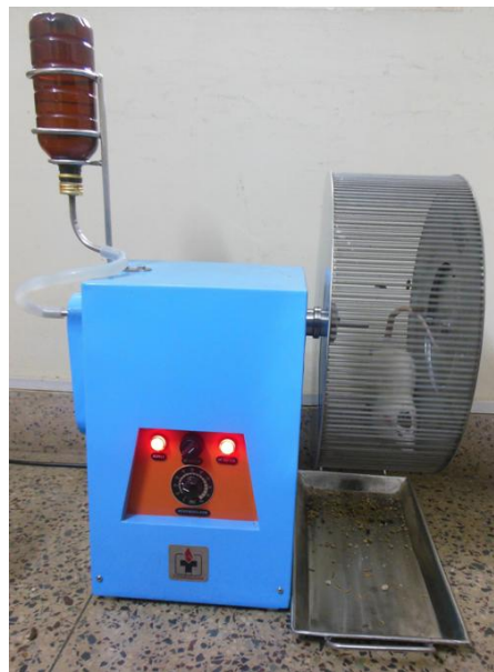
Fig. 11 Custom made rotating wheel for conducting chronic SD in rats
