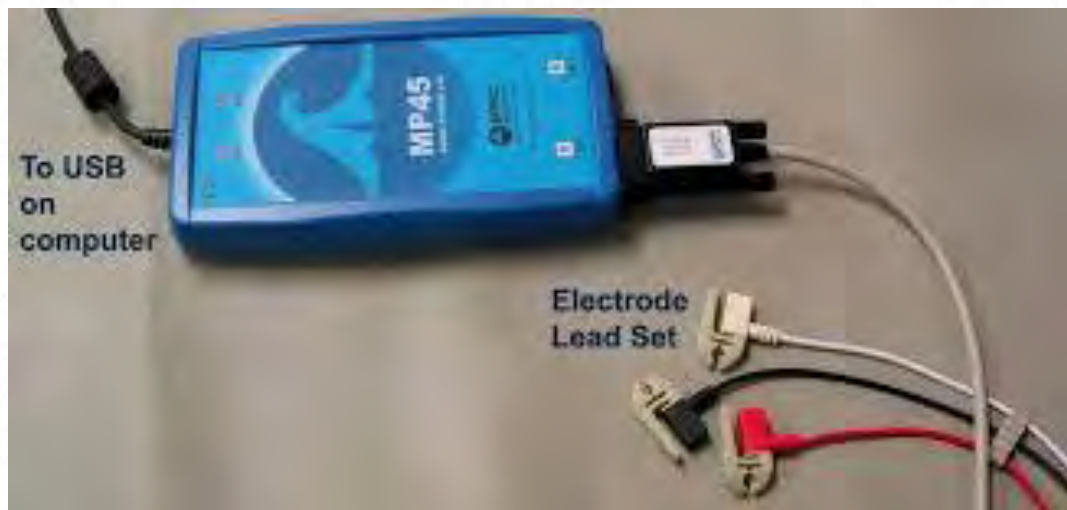
Figure: 5 BIOPAC MP45 machine for ECG recording (Adapted from http://www.oamk.fi/~jjauhiai/opetus/fsk/biopac-ECG%201.pdf accessed on 10/6/2020)
