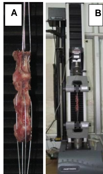
Fig 3- 5: Drilled vertebra bone with stainless steel suture inside ready for tensile test of rabbit IVD (A), INSTRON machine to perform tensile test (B)
