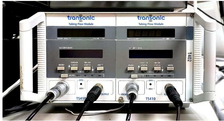
Figure 5.8.b: Transit time Flowmeter. [Transonic Systems Inc., Ithaca, NY]
