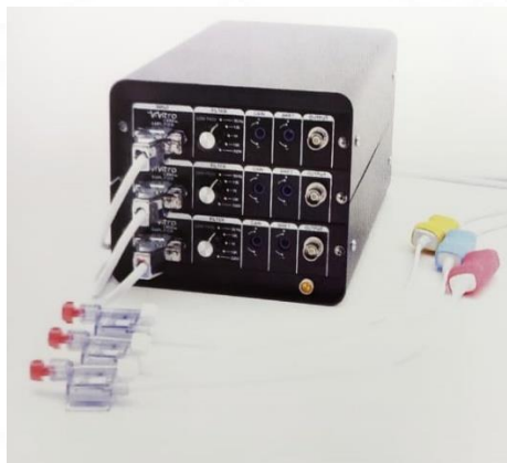
Figure 5.9: Pressure Transducer (HCMO18). [Vivitro labs Inc. Canada]
