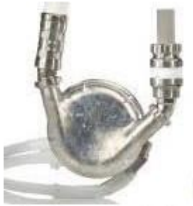
Figure 4.2: First generation pulsatile pump HeartMate XVE. [ResearchGate]
