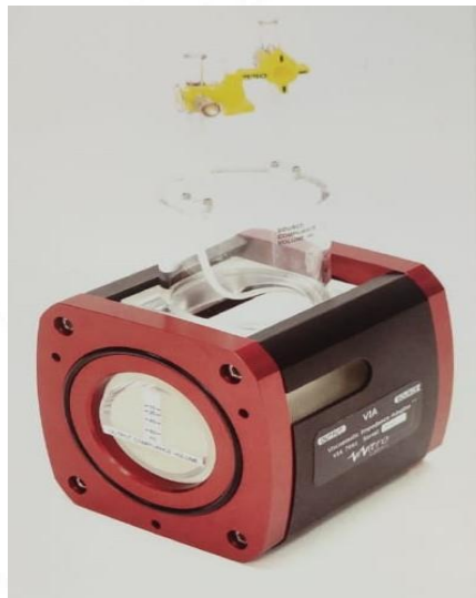
Figure 5.7: Viscoelastic Impedance Adapter (VIA7991). [Vivitro Labs Inc. Canada]
