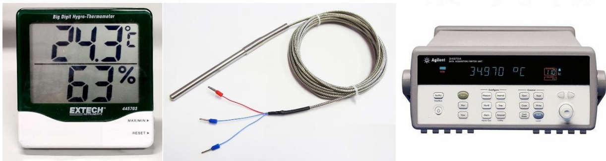
Figure 5.11: Hygro-Thermometer and RTD Temperature probe with Agilent DAS [ Agilent Technologies]
