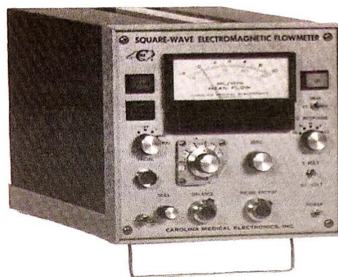
Figure 5.8.a: Electromagnetic Flowmeter [EM Flowmeter, Carolina Medical Electronics, Inc., NC]
