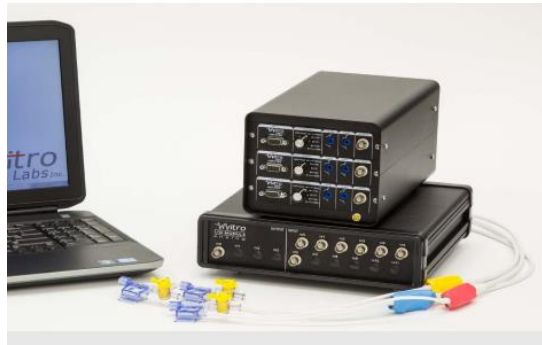
Figure 5.5: Vivitro Data Acquisition system [Vivitro labs Inc. Canada]
