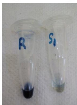
Figure 53: Kaiser test results of peptide synthesis: R represents reference and S represents sample, In R - resin beads after Fmoc deprotection showed blue colour indicating the exposure of amino groups reacting with ninhydrin in Kaiser test. In S – resin beads showing white colour upon reaction with ninhydrin indicates the complete coupling of incoming amino acids with the deprotected previous amino groups.
