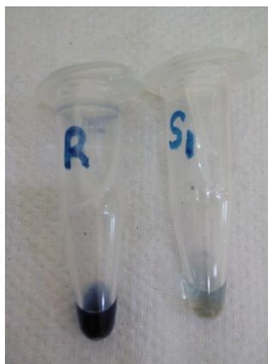
Figure 78: Kaiser test results of peptide synthesis: R represents reference and S represents sample, In R - resin beads after Fmoc deprotection showed blue colour indicating the exposure of amino groups reacting with ninhydrin in Kaiser test. In S – resin beads showing white colour upon reaction with ninhydrin indicates the complete coupling of incoming amino acids with the deprotected previous amino groups.
