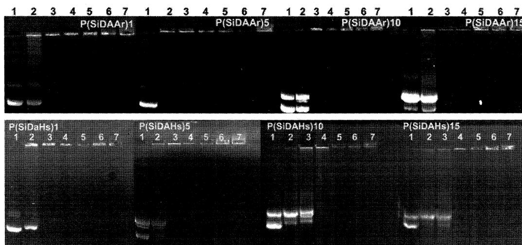
Figure 31: (A) Agarose gel electrophoresis representing pDNA (pGL3 Luciferase reporter vector) binding studies with four P(SiDAAr) n and P(SiDAHs) n derivatives at different w/w ratios. Lane1: pDNA alone, Lanes 2-7 are polymer/pDNA at w/w ratios of 0.25, 0.5, 1, 3, 5 and 10.
