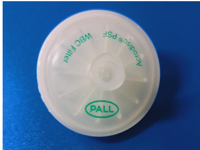
Figure 2: Commercially available leukodepletion syringe filter from PALL Corporation
