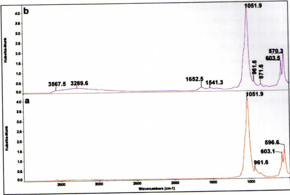
Figure 5.26. Fourier Transform Infrared spectra of HASi remained at the defect site 2 months post-implantation. a) Raw HASi (before implantation) b) HASi 2 months post-implantation.
