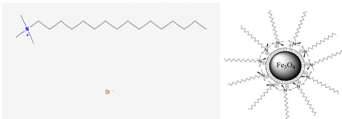
Figure 3 : (a)Structure of CTAB (b)Surface modification of Iron oxide nanoparticle by CTAB(adapted from Kamyar Khoshnevisan et al. 2012)
