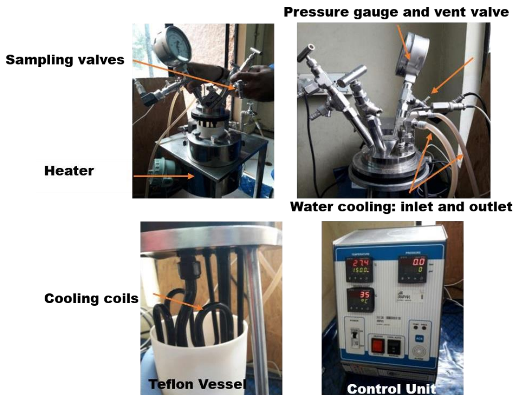
Figure 3.2. Hydrothermal Reactor Parts
