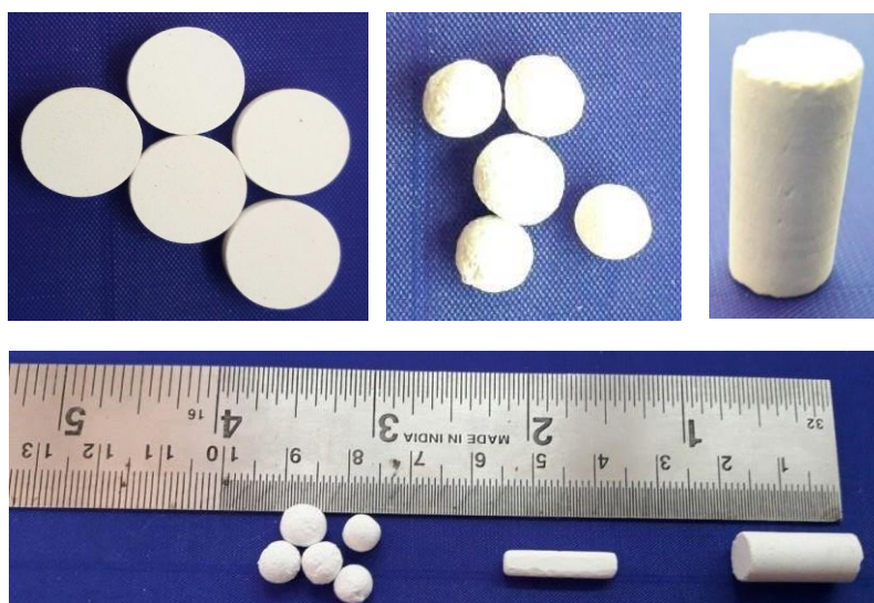
Figure 5.1. Optical micrographs of the calcite preforms for various applications in the study.
