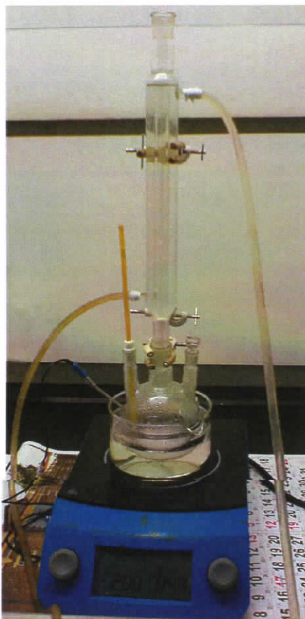
Fig.5: Synthesis of Gelatin Methacrylate monomer (GelMA)
