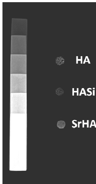
Figure 25 - Radiopacity evaluation of the scaffolds: Radiograph of HA, HASi SrHA scaffolds in comparison to aluminium wedge.
