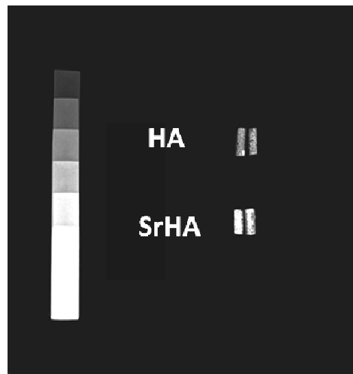
Figure 75 - Radiopacity evaluation: Radiograph depicts the radiopacity of HA SrHA scaffolds in comparison to aluminium wedge.
