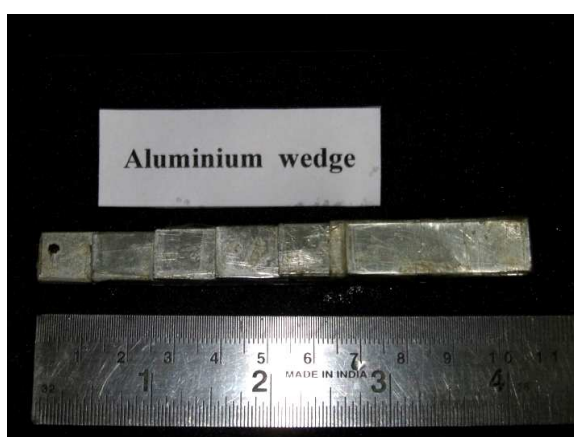
Figure 7 - Aluminium wedge used for quantification of radiopacity of the scaffolds.
