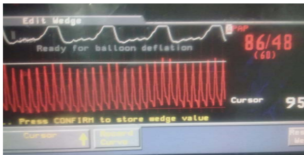
Figure 4: Cursor (white horizontal line) and corresponding pressure value (number in white colour)
