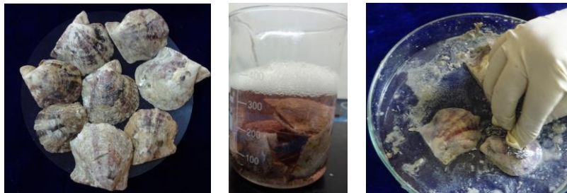
Figure 1. Processing of pearl oyster shells: (a) Shells of Pinctada fucata ; (b) Soaking of shells in acetic acid and NaCl solution and (c) scrubbing the outer prismatic layer.
