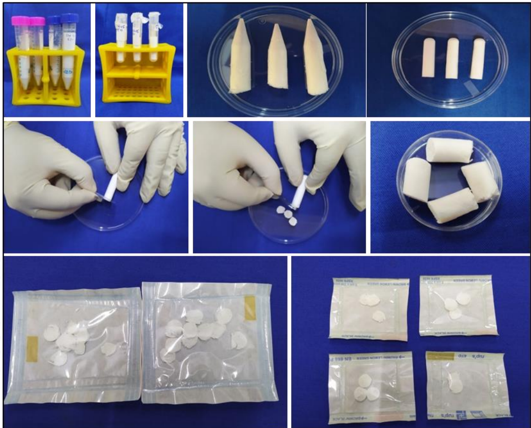
Figure 4.1.1 Fabrication of shell nacre PCL composite scaffolds
