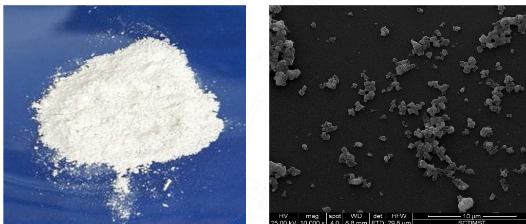
Figure 3.2.5 Shell nacre powder; (a) Macroscopic appearance of shell nacre powder (b) SEM observation of shell nacre powder. Scale bar represents 10 \mu\text{m}
