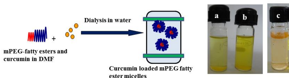
Figure 13. Schematic illustration of preparation of curcumin loaded micelles by dialysis method. (a) Curcumin loaded mPEG laurate micelles (b) Curcumin loaded mPEG linolenate micelles (c) Free curcumin in aqueous media.
