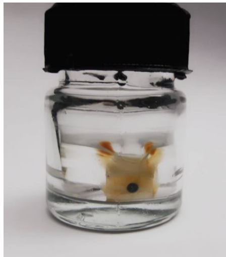
Figure 2.3: Resin embedded bone tissue with implant
