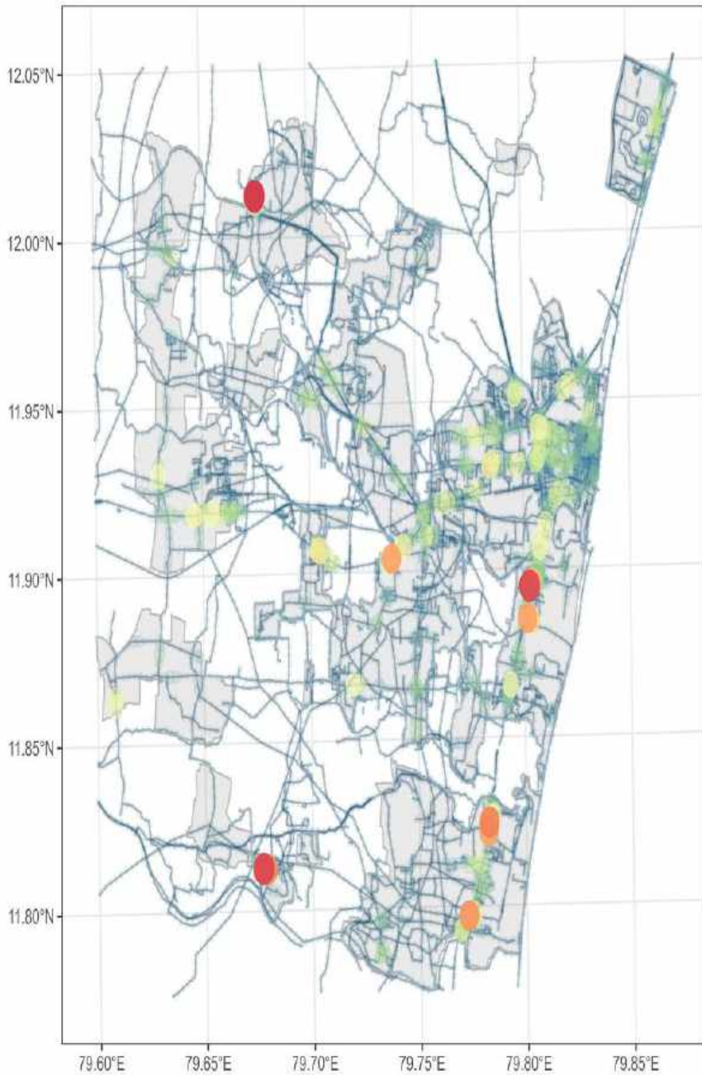
Fig. 4.32. Clusters of ALL road crashes for Half Year (I) of 2018: Mapped by NKDE
