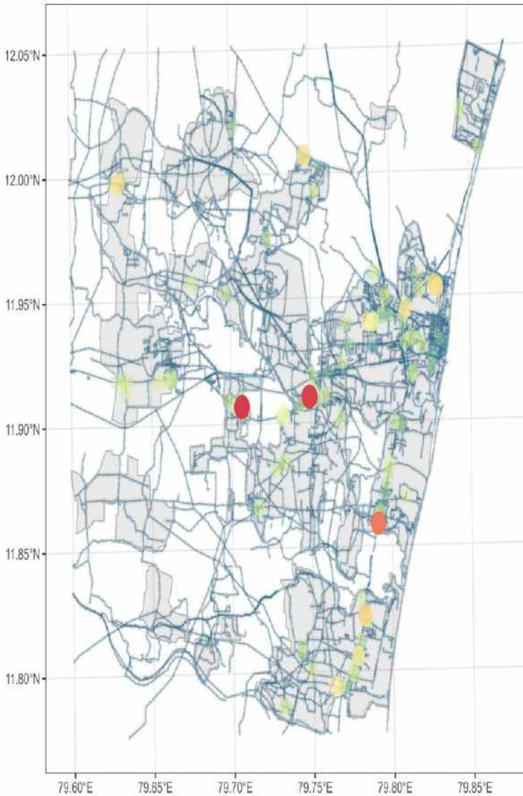
Fig. 4.37. Clusters of FATAL road crash spots for Half Year (I) of 2017 : Mapped by NKDE
