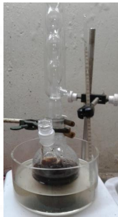
Figure 21. Reaction setup used for the synthesis of EV-g-HR.
