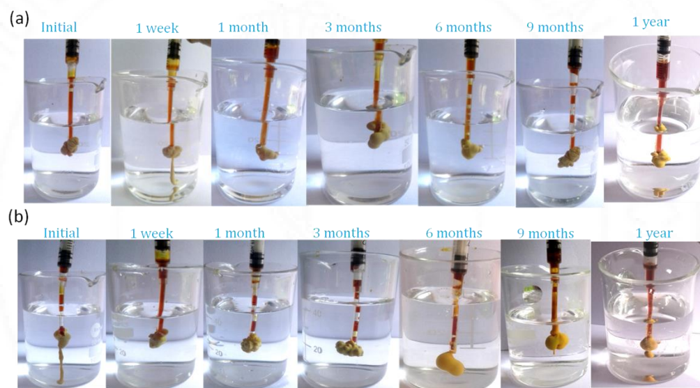
Figure 83. Nature of precipitation of EV27-g-IBHP-120h-35.5% stored at (a) RT, and (b) 37°C
