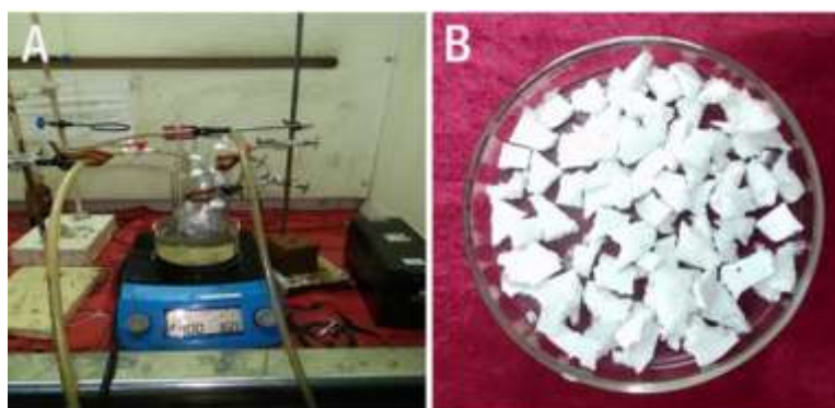
Figure 12. Synthesis of terpolymer PLGC: A) PLGC synthesis set up and B) synthesised terpolymer PLGC.
