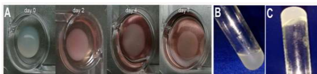
Figure 30. Photographs depicting stability of SFFIBHA hydrogel: A) stability of gel at different time periods, B & C) tilt assay of SFFIBHA hydrogel.
