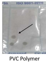
Figure 3 An example of polymer reference material (Positive control material made of PVC)
