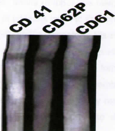
Fig III.A.3 Western blot for CD41, CD62P and CD61 of PD (prepared by 1 IU thrombin activation)
