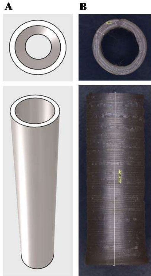
Figure 4.41. (A) CAD image of cylindrical structure. (B) 3D printed PLCL73 cylinder.
