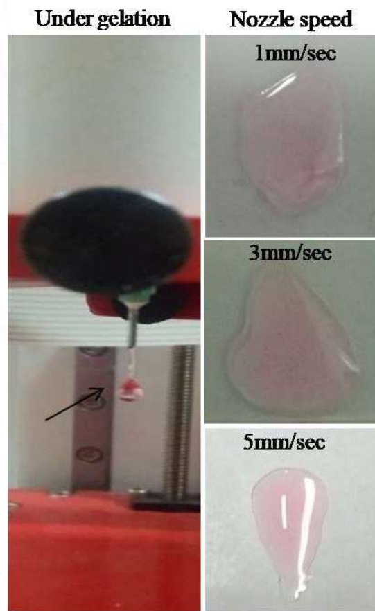
Figure 4.59. CH-HDA 10:1 ratio failed to form continuous filament during extrusion and had low viscosity due to which it did not form any line in line drawing method.
