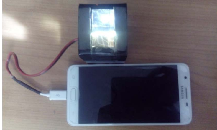
Figure 9: Black reader device which can be fixed onto the smartphone device. The device houses a slit on the top surface to introduce the \mu PAD and 2 LED lights illuminate the black reader box from either side. The LED lights are powered by the phone power using microUSB OTG connection.
