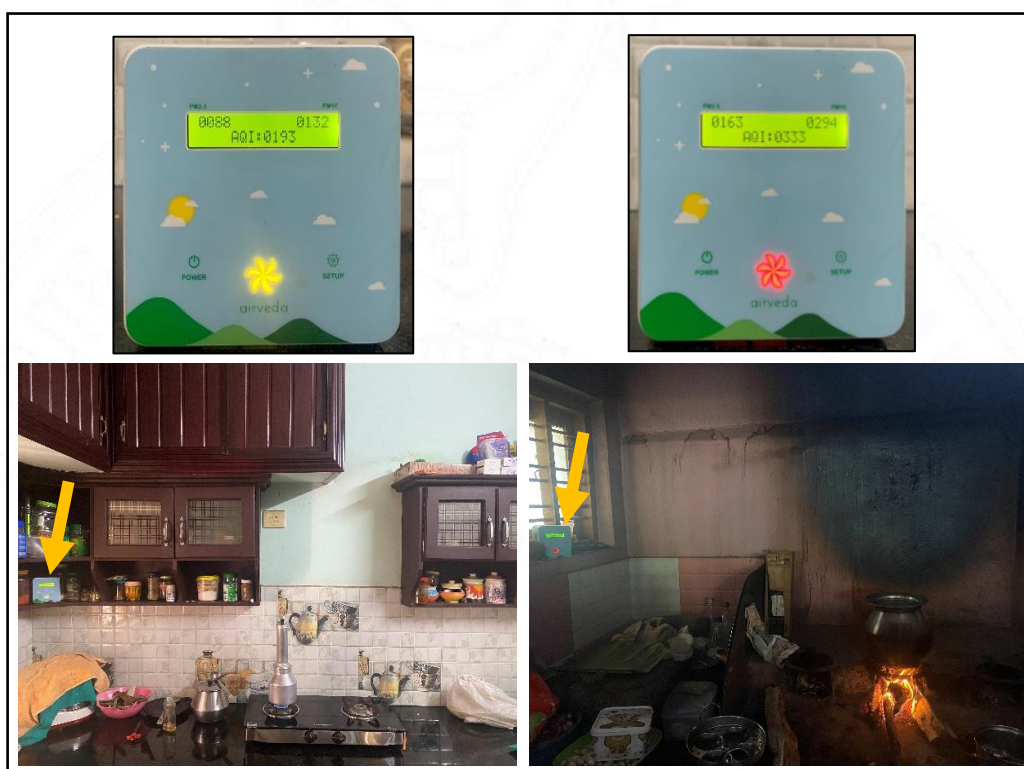
Figure 2.3: Airveda particulate matter monitor and its placement in different kitchen environments
